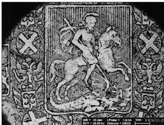
Fig. 2(i) SEM micrograph; high magnification of the 12 rouble coin shows the high quality of the stamping on this coin. A superficial scratch is visible
