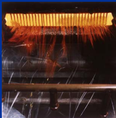
glass fibre bushing in service
