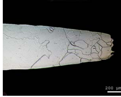
Fig. 13b: Longitudinal section, Ir sheet after creep test at 2000°C/14 MPa
