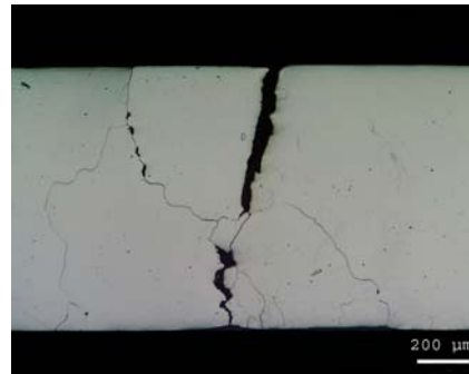
Fig. 11b: Longitudinal section, Ir sheet after creep test at 1800°C/13 MPa
